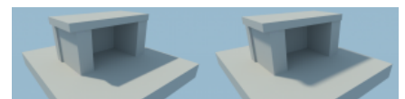
Left: shadow spread = 0.01, right: 0.05. Note how shadows start sharp and get gradually blurrier with distance.
